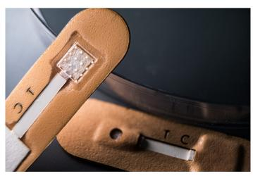
At only 375 microns wide, the microneedles are truly tiny, and do not cause significant pain on insertion. They are hydrophilic, and so easily draw inter-
