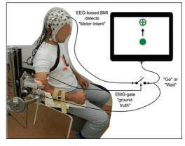
tentions in the EEG signal and moved the arm accordingly. If the intention was not detected, the exoskeleton did not move, which guaranteed the brain's involvement in every motion of the device.
